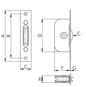
A range of sturdy axle pulleys for sliding sash windows. Sash window axle pulleys are used in traditional rise and fall sash windows to carry the cord attached to the window counter balance sash weight. Typically you will find four in any sash window, two for the top sash and two for the bottom sash. Comes with a 10 year mechanical guarantee.
