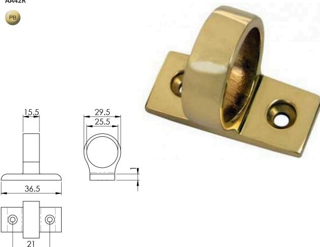
Horizontal fix ring sash lift is a necessary fitting for a sliding sash window in order to open the bottom sash. Two lifts would be fitted, one on either side of the window, in order to open the window with both hands.carlislebrass.
