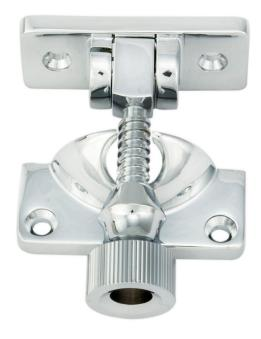
A traditional Brighton pattern sash window sprung fastener. A classic method of fastening and locking sliding sash windows. To lock, pull the sprung toggle arm down and screw the knob into the keep. To unlock, unscrew the knob and the arm will automatically flip up to the vertical position allowing ample clearance between the moving sash windows.
