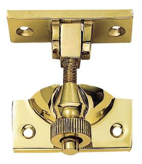
A traditional Brighton pattern sash window sprung fastener. A classic method of fastening and locking sliding sash windows. To lock, pull the sprung toggle arm down and screw the knob into the keep. To unlock, unscrew the knob and the arm will automatically flip up to the vertical position allowing ample clearance between the moving sash windows.
