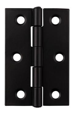
A fixed pin hinge for light domestic use on internal doors. The pin is fixed so cannot be removed. Could be used on an outward swinging exterior door where although the pin is exposed a burglar cannot remove it unlike a loose pin hinge where it can be tapped out and entry gained into the house. Fixed pin door hinges are sometimes also called tight pin door hinges or rigid pin door hinges.
