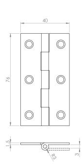
Solid drawn brass hinge traditionally used on cupboards, cabinets and light doors. Comes with a 10 year mechanical guarantee.
