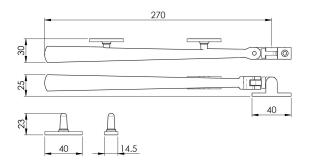
A smart and sturdy solid round-bar window casement stay for timber or aluminium windows. The bar is narrow at the knuckle joint increasing in diameter towards the end resulting in a chunky solid feel. Available in three sizes. The round bar window stay is principally used with the matching round bar window fastener to achieve a consistent style.
