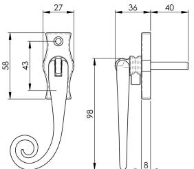
Black antique locking espagnolette fastener. Right or Left hand options. A curly tail window handle which is designed for use on windows that have a multipoint locking mechanism already fitted. The rear spindle connects into the multipoint lock.
