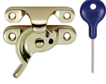
A traditional style of sash window fastener. The operation of the fastener is a simple rotating action for easy opening and closing. The swivelling cam has a rising gradient lip ensuring a firm engagement the harder it is pushed. Locking version available.
