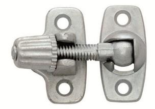
A simple screw down fastener for sash windows. The arm rotates forward to engage the plinth for locking and swivels to one side to allow opening the windows without obstruction.
