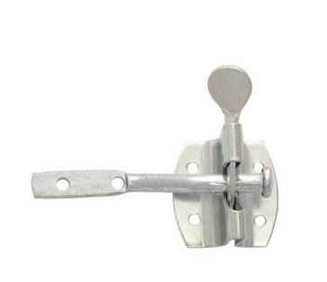
A simple mechanism for closing and securing a gate. When the gate is closed the pin engages and automatically lifts the cam in the latch which then falls in front of the pin securing the gate. The tab of the latch has to be pressed inward to allow the gate to be released.
