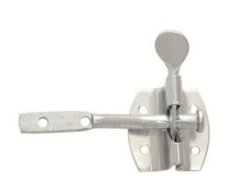
A simple mechanism for closing and securing a gate. When the gate is closed the pin engages and automatically lifts the cam in the latch which then falls in front of the pin securing the gate. The tab of the latch has to be pressed inward to allow the gate to be released.
