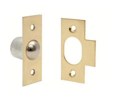
The Bales catch (sometimes referred to as a Ball catch), has a spring loaded ball held within a cylinder attached to a flange. The catch is recessed into the edge of the door while the striker plate is recessed into the jamb. Allows the door to pulled open or closed easily without using an operating handle with a conventional tubular latch .
