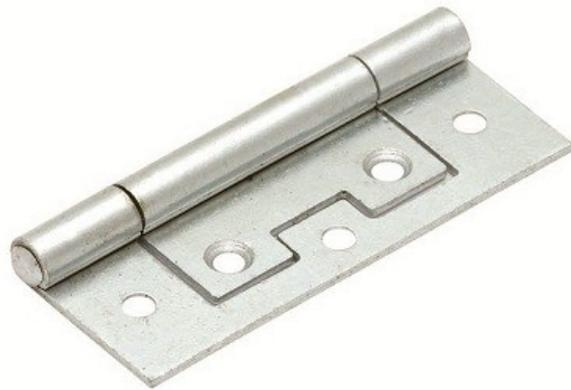
Flush hinge for lightweight applications such as cupboards. Has the advantage over a butt hinge as it fixes directly onto the surface without the need to cut a recess. Also the design allows one leaf to fit inside the other thus taking up less space.
