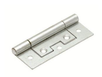
Flush hinge for lightweight applications such as cupboards. Has the advantage over a butt hinge as it fixes directly onto the surface without the need to cut a recess. Also the design allows one leaf to fit inside the other thus taking up less space.
