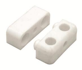
KD Knock down blocks are for making easy joint fixing of cabinet panels. Knock-down fittings are those that can be put together easily, normally using only a screw driver and other basic tools. They are temporary joints although many are used to permanently join together items such as cabinets and other pieces of furniture that are purchased in a flat pack.
