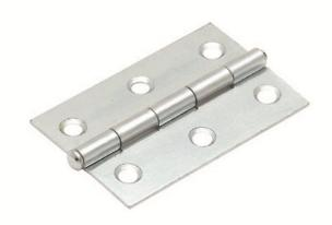
Lightweight loose pin butt hinge. A loose pin butt hinge that has a centre pin that can be easily removed from the barrel to separate the hinge. Also sometimes called removable pin hinges. The advantage of having a loose pin hinge is that the door can be uninstalled without having to remove the hinge from either the door or the door jamb.
