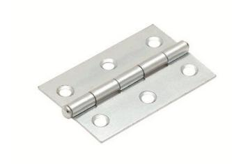
Lightweight loose pin butt hinge. A loose pin butt hinge that has a centre pin that can be easily removed from the barrel to separate the hinge. Also sometimes called removable pin hinges. The advantage of having a loose pin hinge is that the door can be uninstalled without having to remove the hinge from either the door or the door jamb.
