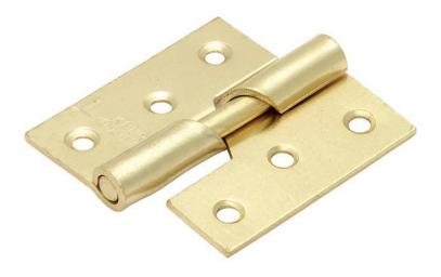
Rising butt hinge left hand version. Rising butt hinges are used to aid doors to self close in such environments as bathroom cubicles. As the door is opened the door rides up the spiral knuckle raising the door as it opens. When the door is released the weight of the door combined with the bevel on the hinged joint causes the door to close by itself in the majority of cases, although this action is not entirely reliable.
