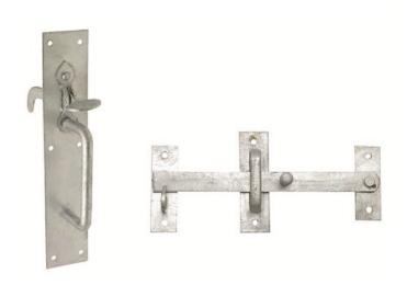
A traditional basic operation gate latch. When the thumb latch is depressed this raises the latch bar on the other side of the gate from its keep allowing the gate to open.
