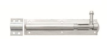
Tower bolt (or barrel bolt). The simple and popular basic door security device. Standard straight barrel bolt. The bolt is slid into the staple and the finger knob is rotated to engage in the housing slot thus locking it in position.
