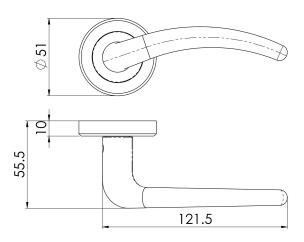
Lever on a concealed fix 2 part screw on round rose. The Luna lever features a smooth shape that is curved and thins out towards the end. This ergonomic design ensures the utmost comfort and ease of use. The chamfered edge concealed fix rose reflects the attention to detail in this range.
