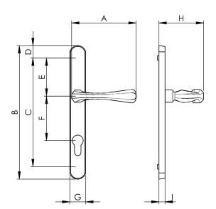
Lever on lock narrowplate for operating a multipoint locking system. Euro profile in either 70mm or 92mm c/c. A smooth round bar lever which expands to a rotund end making this handle very easy to grasp. The handle has fabulous ergonomics fitting comfortably in hand and giving a good positive action in operation.
