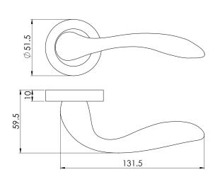
Lever on concealed fix 2 part screw on round rose. The ergonomic contours of the lever blend seamlessly with the hand offering comfort as well as stylish looks. Comes with a 10 year mechanical guarantee and is Fire door rated. Suitable for domestic and commercial use.
