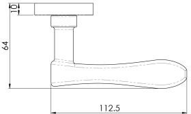
Lever on concealed fix 2 part screw on round rose. A robust curved lever which fits neatly in the hand and provides a comfortable and positive action in use. Comes with a 10 year mechanical guarantee and is Fire door rated. Suitable for domestic and commercial use.
