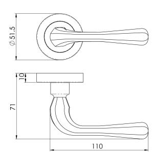
Lever on concealed fix 2 part screw on round rose. A smooth round bar lever which expands to a rotund end making this handle very easy to grasp. The handle has fabulous ergonomics, fitting comfortably in the hand and giving a good positive action in operation. Comes with a 10 year mechanical guarantee and is Fire door rated.
