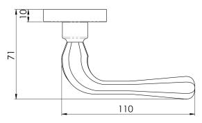
Lever on concealed fix 2 part screw on round rose. A smooth round bar lever which expands to a rotund end making this handle very easy to grasp. The handle has fabulous ergonomics, fitting comfortably in the hand and giving a good positive action in operation. Comes with a 10 year mechanical guarantee and is Fire door rated.
