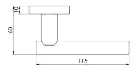
Lever on concealed fix 2 part screw on round rose. A plain straight round bar lever which is easy to grasp and operate comfortably. Its minimalistic lines will look good in any environment. Comes with a 10 year mechanical guarantee and is Fire door rated.
