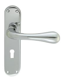
Lever on lock backplate. Standard profile 57mm c/c. Plain, shaped backplate with rounded ends. A smooth round bar lever which expands to a rotund end making this handle very easy to grasp.
