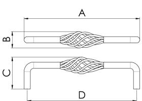
Steel cage fixed pull handle. A D type pull handle with an intricate central oval cage giving this handle comfort and substance to grip.
