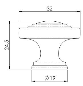
A traditional round ringed pattern knob on a stem rose making it easy to grasp. Provides a comfortable feel and good torque when opening doors and drawers.carlislebrass.
