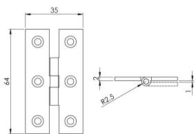
H pattern hinges are classically used on traditional cabinets with the hinge exposed. Placed on the outside of the door the hinge is highly visible and becomes a decorative part of the built-in furniture.
