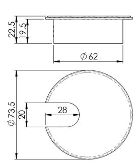
A recessed heavy pattern cable tidy adding a quality touch to perfectly cover any drilled holes for cables in worktops and desk tops.
