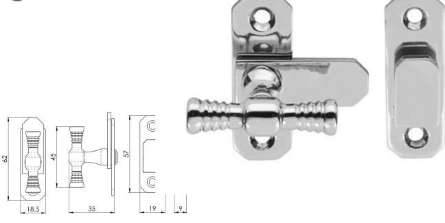
T-handle window fastener. Simple turning action of the ringed handle will fasten casement windows together when they are in the closed position. Not suitable as a one and only form of window locking. Can also be used in general purpose locking for cabinets, doors.
