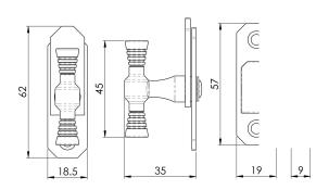
T-handle window fastener. Simple turning action of the ringed handle will fasten casement windows together when they are in the closed position. Not suitable as a one and only form of window locking. Can also be used in general purpose locking for cabinets, doors.
