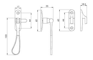
A plain spoon ended pivot-reversing non-locking casement fastener, one of the most commonly used fasteners for traditional timber windows. It operates with either a mortice or hook plate and is reversible. Not suitable for use on weather stripped windows. Comes with a 10 year mechanical guarantee.
