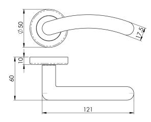
Lever on a concealed fix 2 part screw on round rose. A contemporary arched round bar lever on rose. Part of the Serozzetta Zin lever designer collection. Comes with a 10 year mechanical guarantee and is fire door rated.
