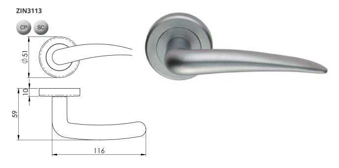
Lever on a concealed fix 2 part screw on round rose. A straight tapering lever on rose. Part of the Serozzetta Zin lever designer collection. Comes with a 10 year mechanical guarantee and is fire door rated.
