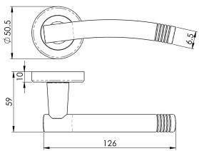
Lever on a concealed fix 2 part screw on round rose. A slightly arched round bar lever with a ringed feature at the end of the handle. Part of the Serozzetta Zin lever designer collection. Comes with a 10 year mechanical guarantee and is fire door rated.
