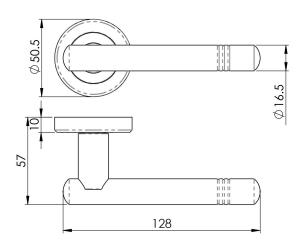
Lever on a concealed fix 2 part screw on round rose. A straight round bar lever with a ringed feature towards the end of the handle. Part of the Serozzetta Zin lever designer collection. Comes with a 10 year mechanical guarantee and is fire door rated.
