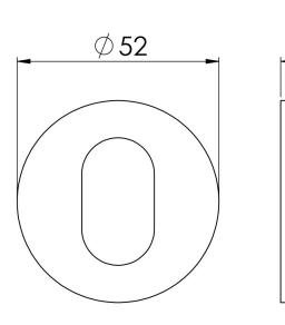
Escutcheon on a concealed fix press on rose. Options Blank, Euro, Lock and Oval. Comes with a 10 year mechanical guarantee and is Fire door rated. Part of the Aluminium range.
