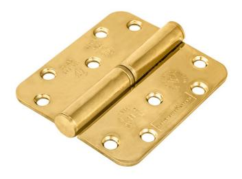
Square or Radius options in Left or Right handed variants. (Max Load 80kg). Lift-off hinges, allow a door to be removed without unscrewing the leaves themselves. This improves access and allows large items to pass through freely and alleviates damage to the door itself.
