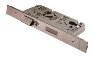
Din Euro Profile Escape Lock 60mm. Square and Radius options. The Latch bolt has the Easi-T reverse function to save undoing the case so it can be reversed in seconds. British Standard BS EN 12209 and 179 Rated lock used as a matter of course by the national house builders.
