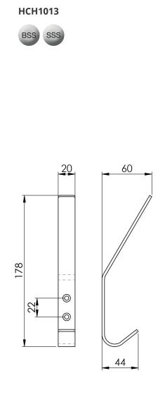
A robust flat bar hat and coat hook with smooth radiused corners for safety and two central fixing points providing a secure fitting. Part of the Steelworx Stainless steel range offering a flawless finish. Fire door rated. Suitable for domestic and commercial use.
