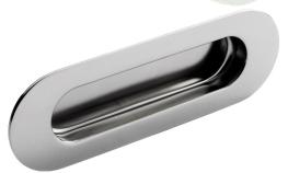
120mm x 40mm A radius shaped low profile flush pull which is used mainly on sliding doors. The main cup is recessed back into the door to leave a flush appearance. For use on doors, wardrobes or cupboards. Part of the Steelworx Stainless Steel range.
