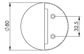
Large shielded half moon shaped door stop with a substantial rubber buffer to protect doors. Small version available. Part of the Steelworx Stainless Steel range. Comes with a 10 year mechanical guarantee.
