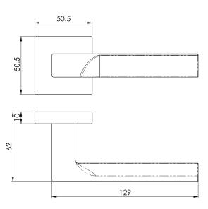
Lever on concealed fix square rose. A flat bar lever initially retaining its square appearance emanating from the stem then delicately forming to a thinner angular blade. The angle of the lever is so ergonomic the hand and thumb conform naturally to provide a comfortable and assured grip. Comes with a 10 year guarantee.
