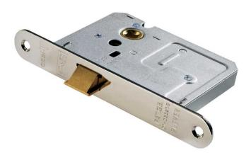
Contract Upright Latch. Square or Radius Forend, 64mm and 76mm options. The Latchbolt has the Easi-T reverse function to save undoing the case so it can be reversed in seconds. Certified to BS EN 12209.
