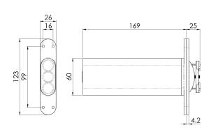
Door closer suitable for light or medium weight doors. The main body fits into the door but this can be reversed where required for narrow stile doors when the hydraulic housing can be fitted into the wall frame. Comes with a 2 year mechanical guarantee and is fire door rated. Maximum Door width 940mm, maximum weight 80kg, angle of opening maximum 110 degrees, suitable for Left or Right Hand use.
