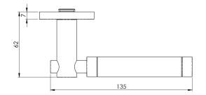
Lever on a concealed fix threaded rose. A stylish round bar sectional lever with a dual finish which accentuates the components in this unique modern design. Part of the Steelworx range in grade 304 Stainless Steel. Comes with a 10 year mechanical guarantee and is Fire door rated.
