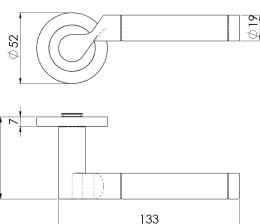
Lever on a concealed fix threaded rose. A stylish round bar sectional lever with a dual finish which accentuates the components in this unique modern design. The shaped front of the lever creates a natural thumb grip and makes it comfortable to hold and use. Part of the Steelworx range in grade 304 Stainless Steel.
