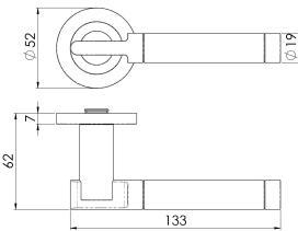
Lever on a concealed fix threaded rose. A stylish round bar sectional lever with a dual finish which accentuates the components in this unique modern design. The shaped front of the lever is inset into the stem neck. Part of the Steelworx range in grade 304 Stainless Steel.
